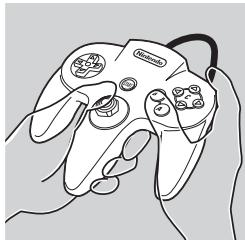
By holding the controller like this, you can operate the Control Stick freely with your left thumb. Using your right thumb, you can easily access the A-, B- or C-Buttons.
